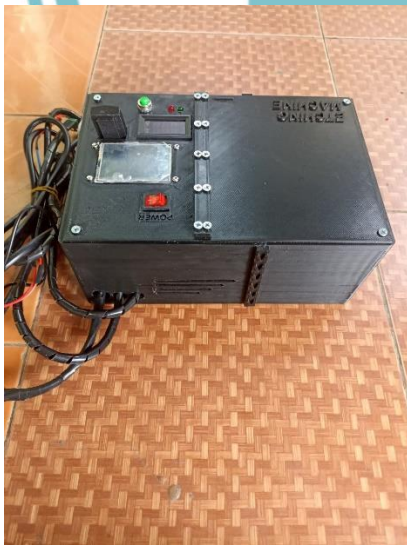
Gambar Enclosure (Box kontrol)
