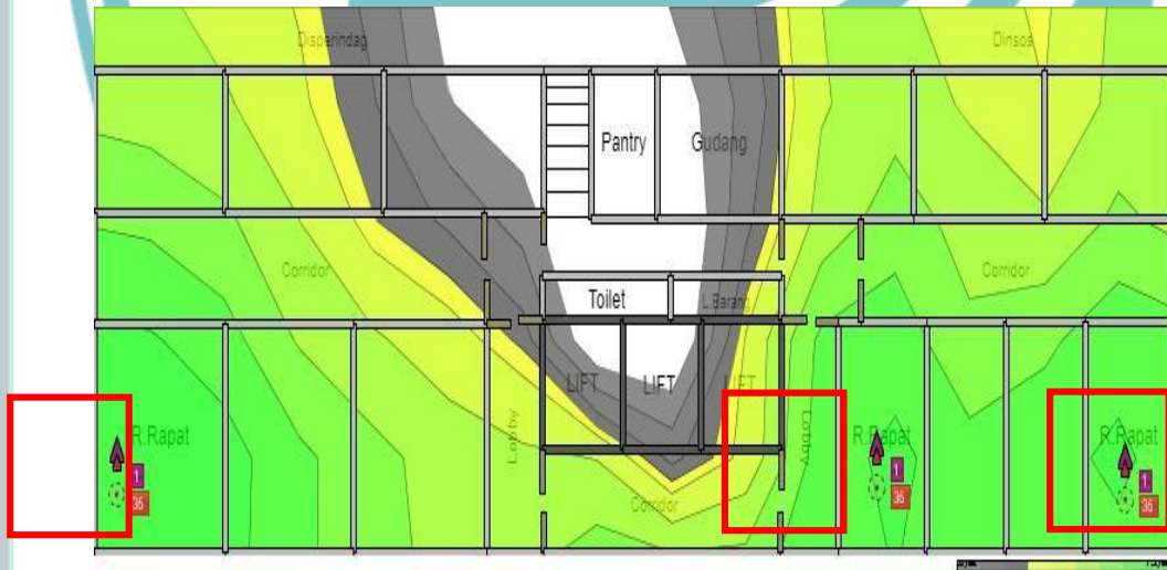
Lampiran 6—Hasil Pengujian Coverage Area Lantai 6
