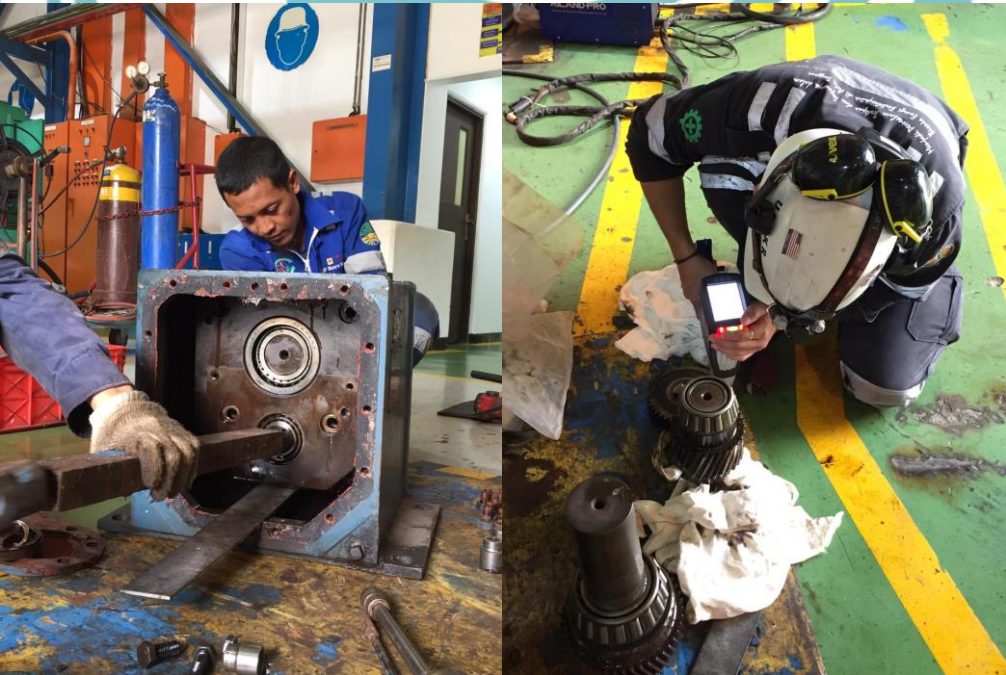
Gambar 3 Preventive Maintenance - Cleaning Mechanical Seal
