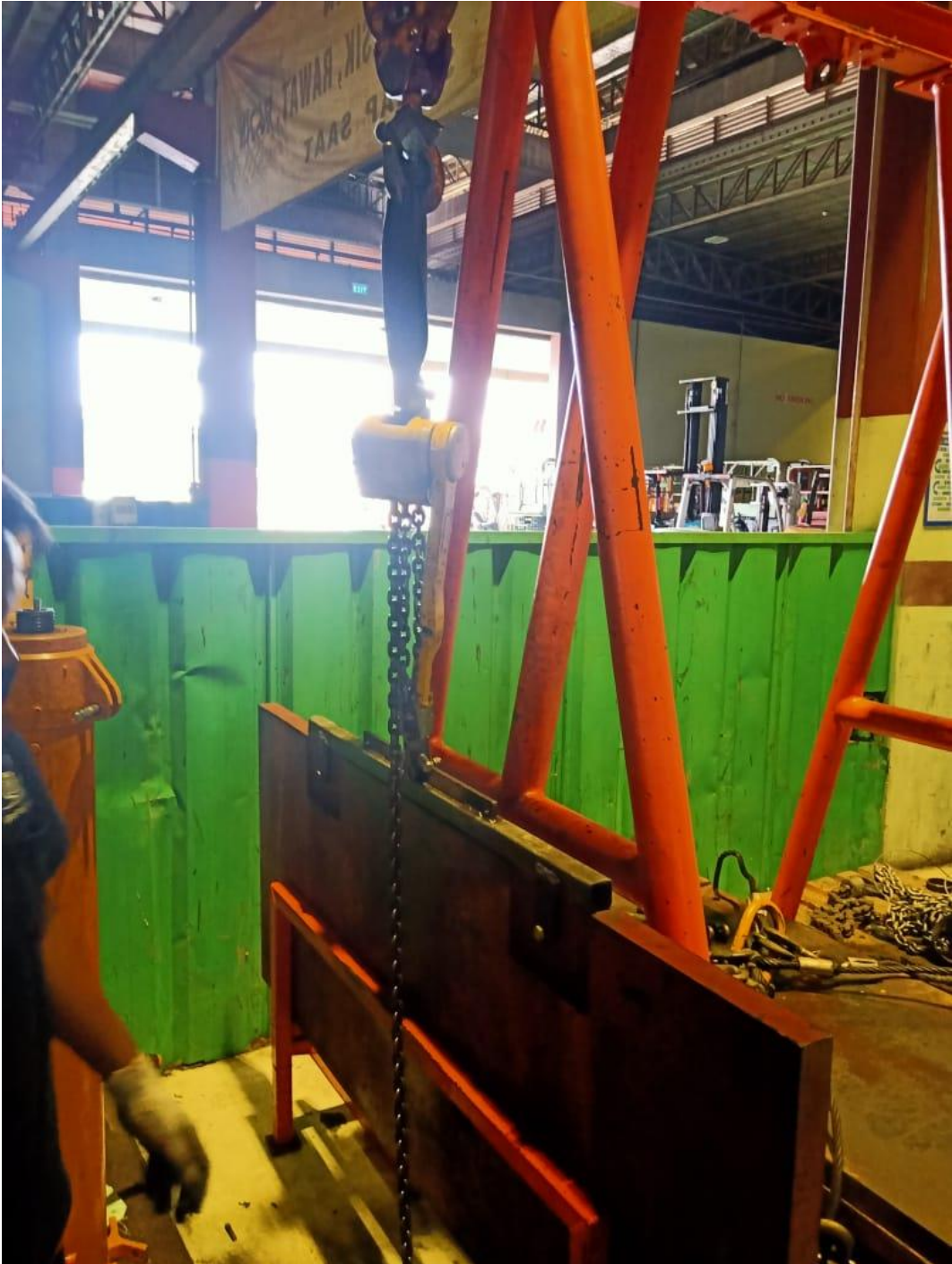
Lampiran 7 : Proses Test Load Chain Hoist
