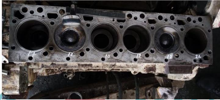
Gambar 2. 8 *Cylinder Block*
