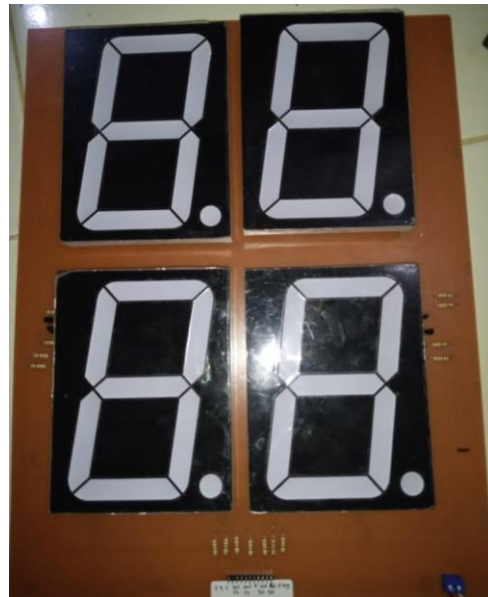
Hasil Realisasi Layout PCB Seven Segment
