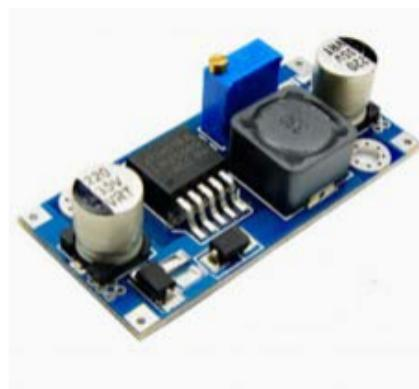
LM2596 DC to DC step down regulator, adjustable +1.23 to 35vdc output, 2A. Ideal for battery operated projects requiring a regulated powersupply.
