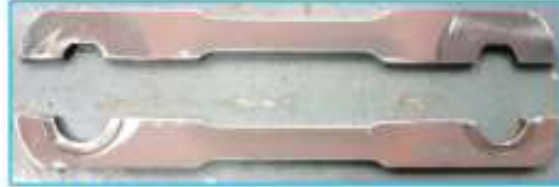
Gambar 20. Sample Chain Link Approne Conveyor Sebelum Uji Tarik
