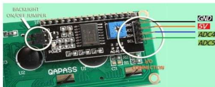
LCD display to Arduino wiring.
