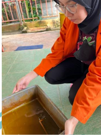
Proses Meng-etching PCB
