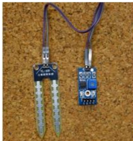
The sensor has a built-in potentiometer for sensitivity
