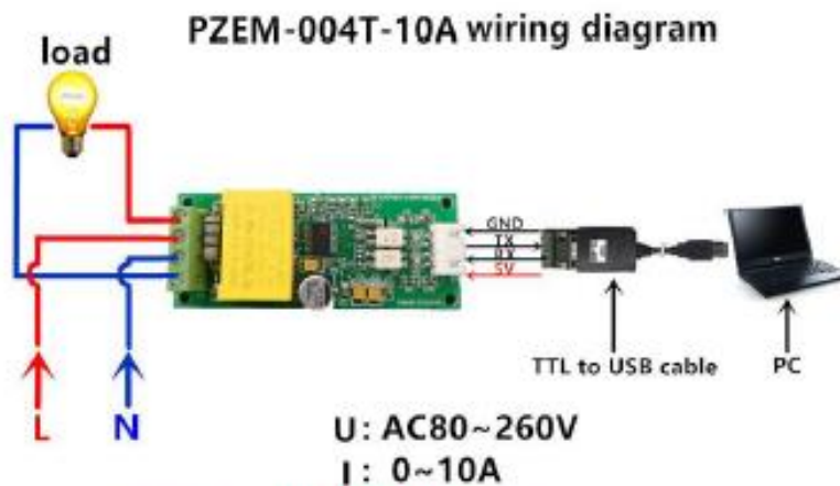
Picture 4.1 PZEM-004T-10A wiring diagram
