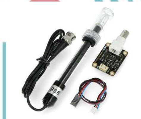
Gambar 2.6 Sensor *Electrical Conductivity*
