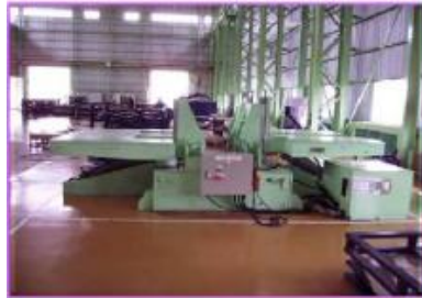
TURN OVER MACHINE Maker : TOYO IDEC Co. Ltd Capacity : 7 Ton
