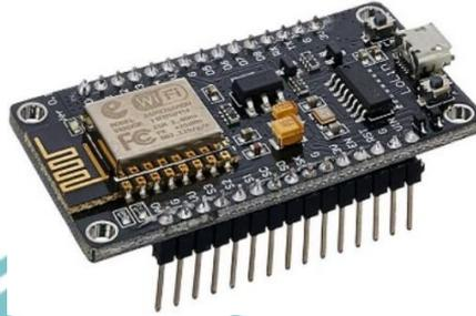
Gambar 2.7 NodeMCU ESP8266
