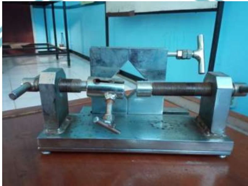
Gambar 1. 1 Gambar Prototype Alat Bantu Pelepas Universal Joint
