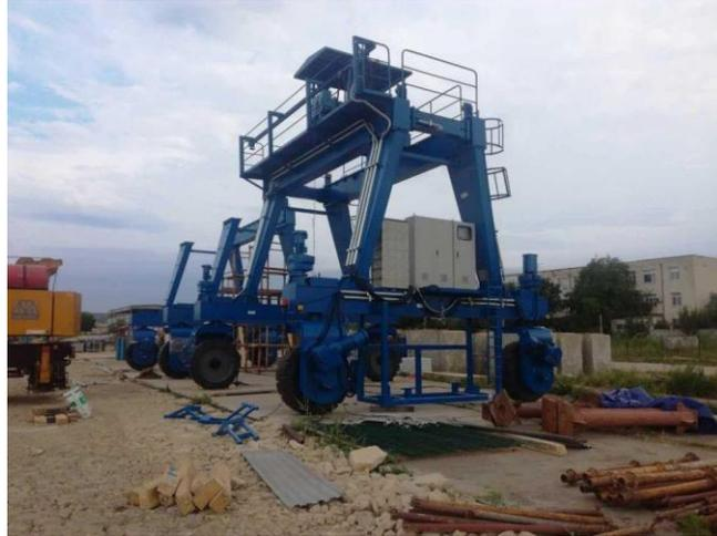
Gambar 2.3. *Rubber Tyred Gantry Crane (RTG Crane)*
