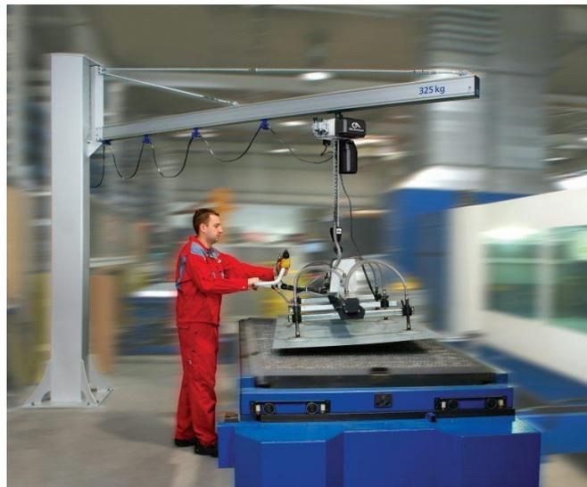
Gambar 2.6. Workstation Crane / Aluminium Light Crane
