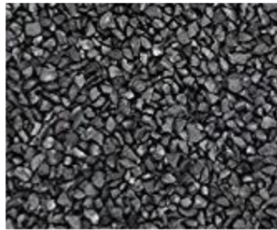
Figure 1 Steel grit G25 particle (particle size: 0.71 – 1.19 mm)
