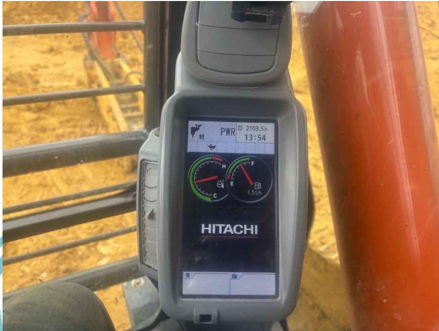
Gambar 4.2 Jam Operasi Excavator
