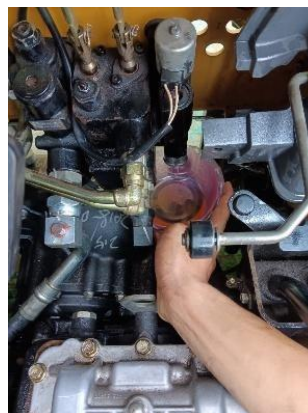
Gambar 3 Internal Leakage Test
