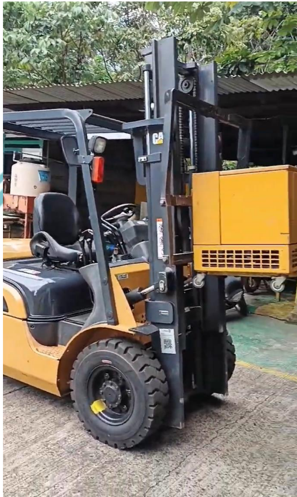
Lampiran 2. Pengambilan Data Tilt Cylinder dan Internal Leakage
