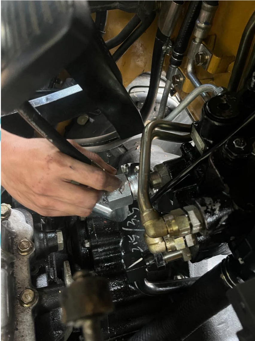
Lampiran 1. Pengecekan Control Valve
