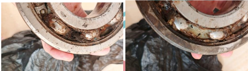
Lampiran 1 Kondisi Ball Bearing 6311
