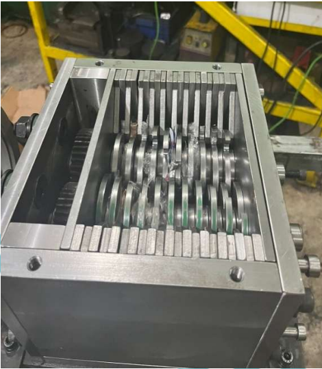
full assembly shredder box
