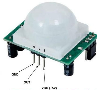
Gambar 2.3 Sensor Passive Infrared Receiver (PIR)
