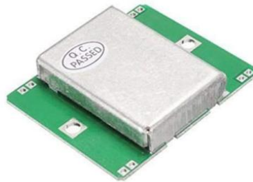
Gambar 2.2 Sensor Radar Doppler HB100
