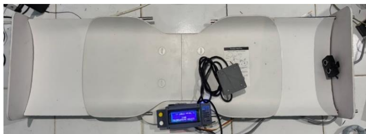
Gambar 4.19 Set up sensor rotary encoder alat antropometri
