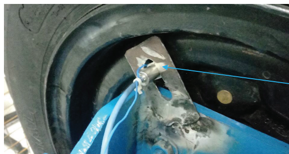
Fig. 3. Optimal position of the thermocouple sensor in the drum brake
