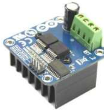
Gambar 2. 8 Driver Water Pump
