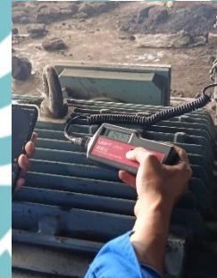
Gambar 14 Pengukuran Vibrasi Gearbox BC 5B
