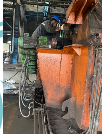
Gambar 5.8 Greasing Motor Roller Screen B
