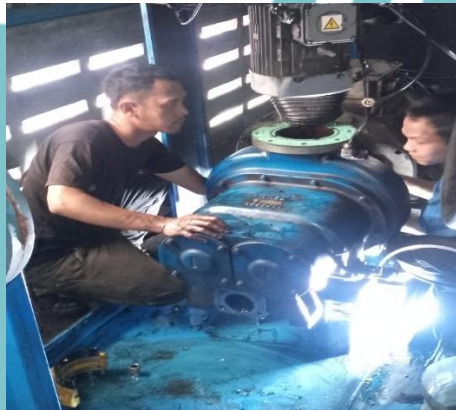
Gambar 4 Disassembly Screw Kompresor Plant Machining
