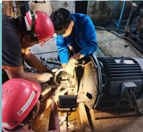
Gambar 7 Disassembly Screw Kompresor Plant Plastik
