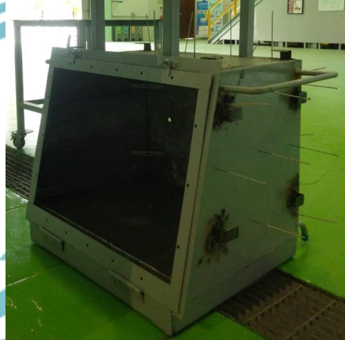
Proses Insulasi Oven
