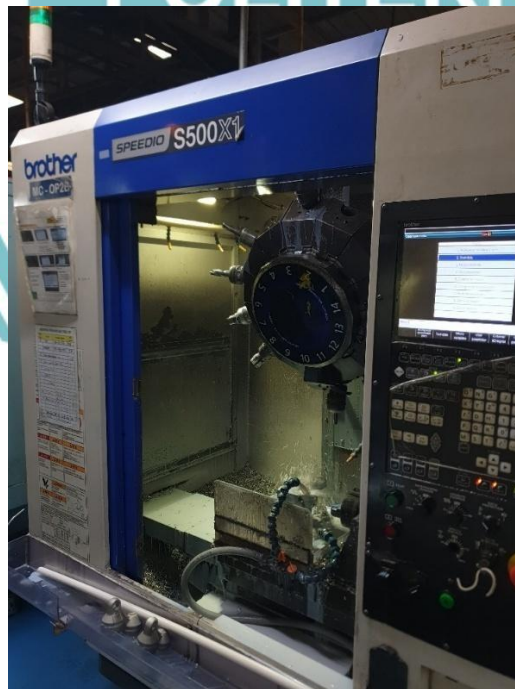
Lampiran 2 Mesin CNC Brother Speedio S500X1 Saat Pintu Terbuka
