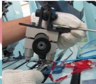
Gambar 1. 2 Proses setting alat uji steering handle durability
