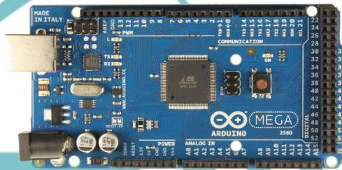
Gambar 2. 2 Arduino Mega 2560
