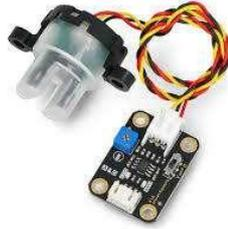
Gambar 2. 4 Sensor *Turbidity* DFRobot
