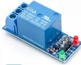
Gambar 2. 16 Relay 1 *channel*
