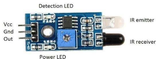
Gambar 2.10 Sensor Infrared
