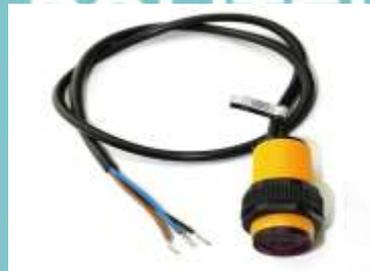
Gambar 2. 5 Sensor Infrared
