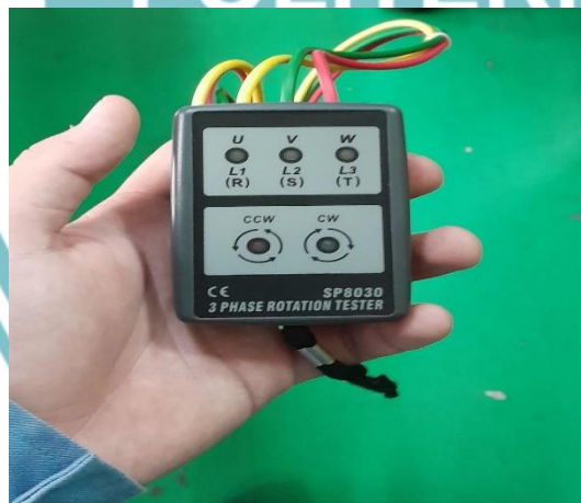
Gambar 4. 6 Pengetesan Phasequence 3 Rotation
