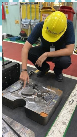
lampiran 3 pengecekan crack cavity fix
