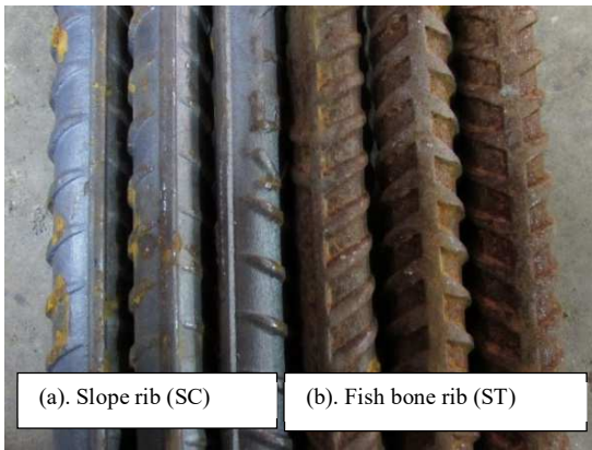
Fig. 3 Deform bars (a). slope rib (SC), (b). fishbone rib (ST)
