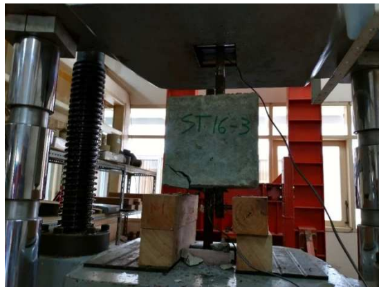
Fig. 4 The setting of pullout testing using UTM
