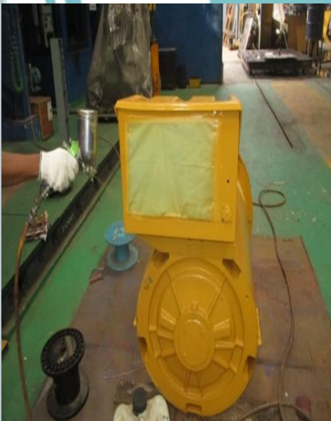
Proses pengecatan body generator
