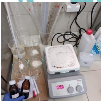
Magnetic hotplate stirrer merk DLAB, gelas laboratorium, thermometer, pipet dan aluminium foil
