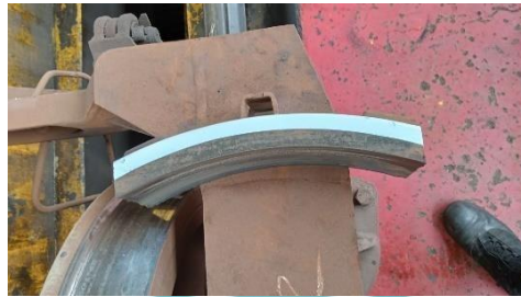
(Marking maksimum keausan Block Break)
