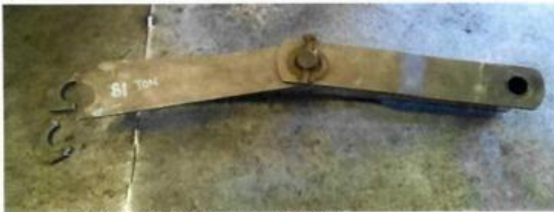
AFTER TEST BREAK 81 TON (794,6kN)
