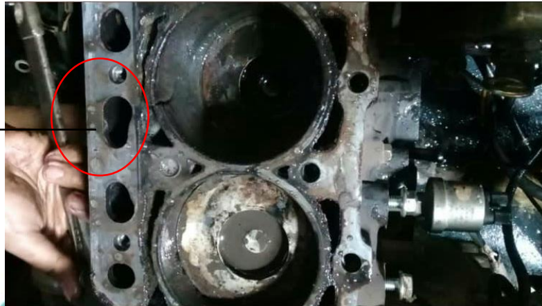
Gambar 1. 1 Kerusakan Cylinder Liner
