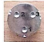
Fig 2. Specimen After Indentation
