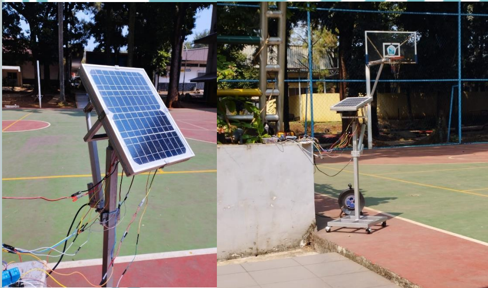
Gambar 6. 1 Rangkaian Panel Surya Solar Tracker dan Heatsink Cooling Fan
