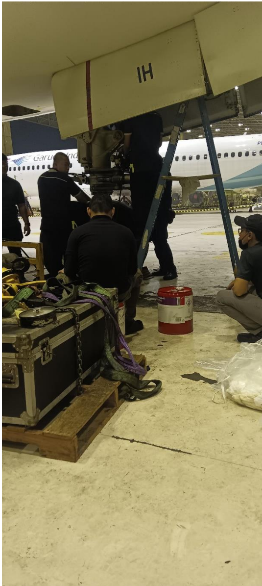
Gambar 4.2.2 Servicing NLG Shock Strut
