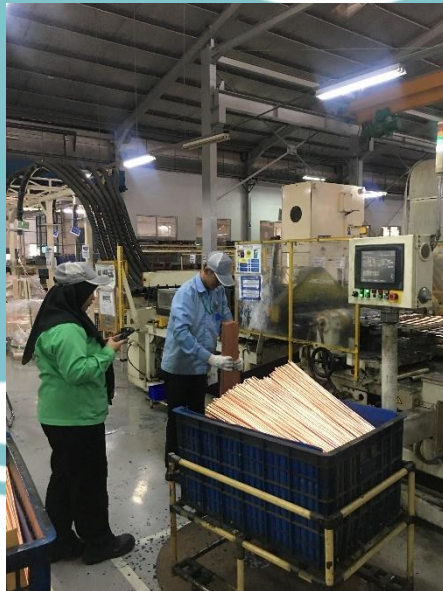
Proses pengambilan data cycle time pada mesin hairpin bending Section 2 Manufacturing 2 (Evacond)
