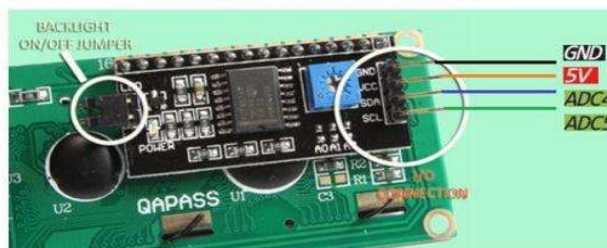
LCD display to Arduino wiring.
