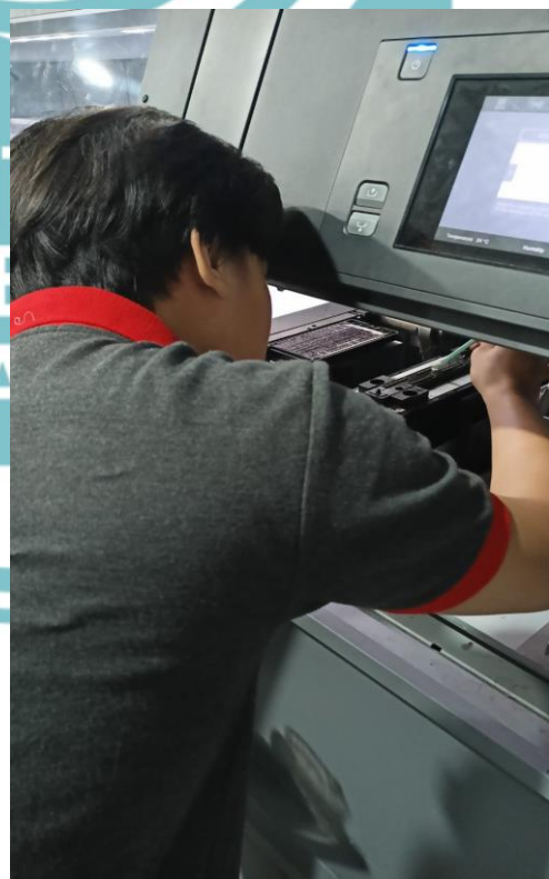
Melakukan Preventive Maintenance mingguan cleaning mesin Print Epson 10030
