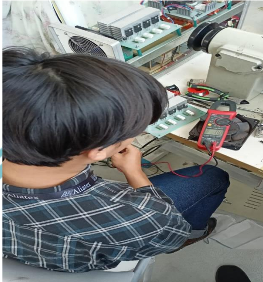
Memeriksa board transistor mesin ultrasonic sewing
