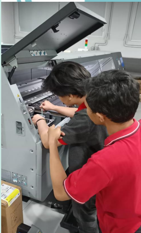
Melakukan Preventive Maintenance mingguan cleaning mesin Print Epson 10030
